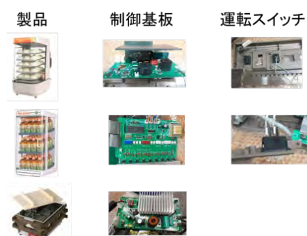
Fig.6-11 Expected ignition source in equipment
